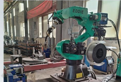
Welding by robot
