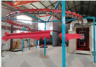
Automatic spraying line
